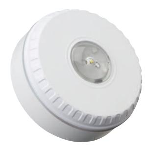
The Solista LX Ceiling has a unique lens design that distributes the light in a cylindrical shape to achieve the required illumination specified by EN 54-23. Designed for installation at a height of up to 3m and with a discrete appearance, the device is ideal for a variety of applications, including bedrooms, bathrooms and toilets.
